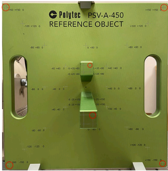
Fig. A1. Details of the reference object and points marked by red circles for calibration purposes.
