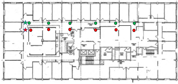
Figure 9: Floor plan for power draw experiments. Star designates the peer attached to the Monsoon power meter. Dots designate the other peer in LoS (green) and nLoS (red).
