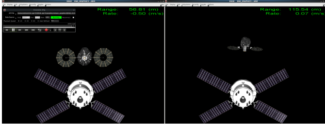
Fig. 11: NASA spaceflight simulation without (left) and with (right) PCSPoof. PCSPoof caused a significant deviation in the vehicle’s flight path, which prevented docking.
