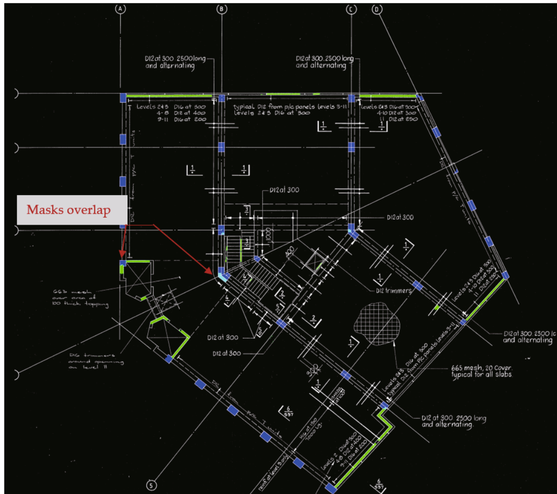
Fig. 14 Overlay of the prediction on the structural drawing
