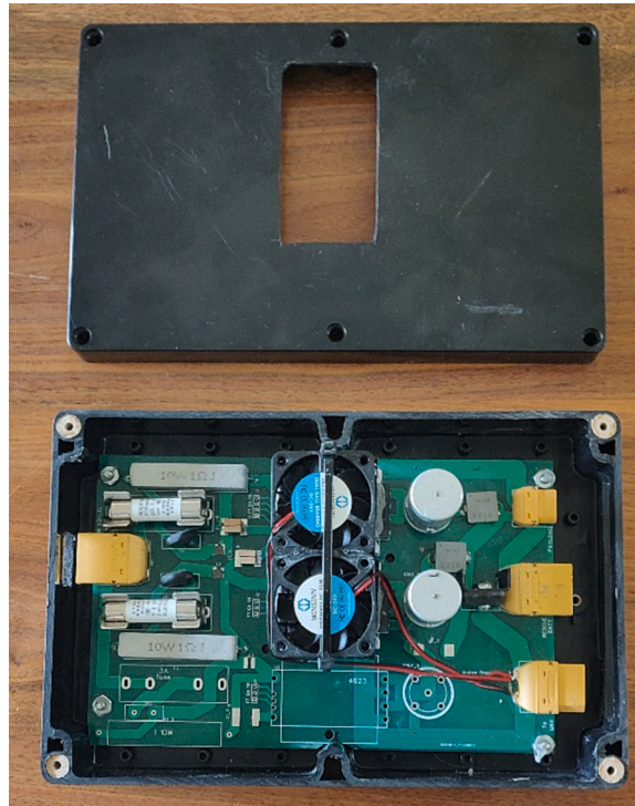
Fig. 14. Completed top power module with room for third DC-DC converter. Lid screws in place.
