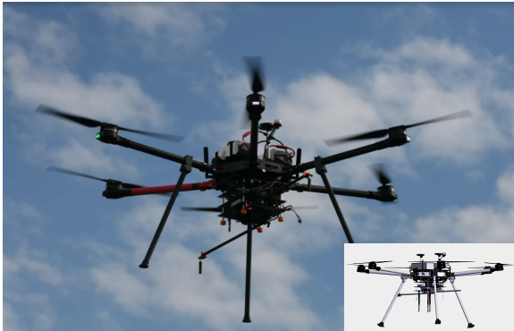
Figure 3: Large AERPAW Multicopter (LAM6) with Portable Node and CAD model.
