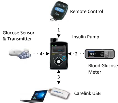
Fig. 1: A real time insulin pump system
