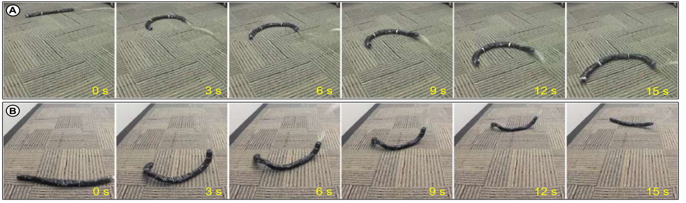
Fig. 10. The SRS pose progression for (A) Planar and (B) Spatial rolling gaits at 3 bar – 0.50 Hz.
