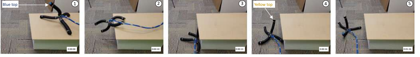
Fig. 9: Topple proof demonstration. (1) Robot moves with a blue marker at the tip (i.e., end). (2) Falling. (3) Remap the limb configuration according to the Yellow limb. (4) Push away from the obstacle. (5) Moves forward as normal.
