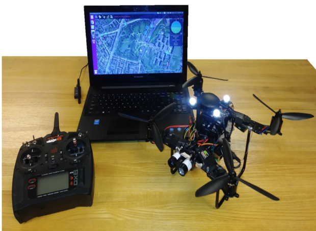
Fig. 2 The developed UAV and its ground station
