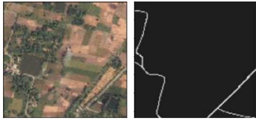
(a) Satellite image & ground-truth label (extracted roads).
