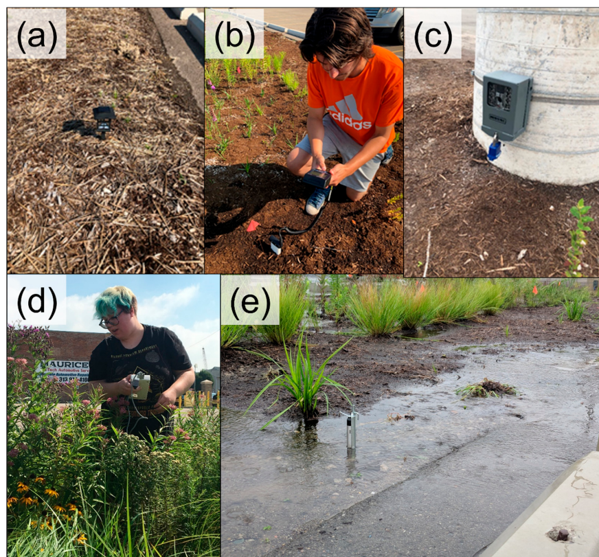
Figure 4. Site photographs of the field survey and instruments illustrating (a) iButtons in solar-light housing, (b) weekly soil moisture measurements, (c) a phenocam mounted on south lamppost, (d) weekly stomatal conductance measurements, and (e) a pressure transducer at one of the inputs to the bioswale after a rainstorm.
