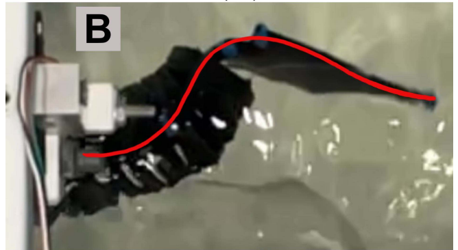
Fig. 5. (A) Tracked shape of 38.71 cm 2 triangle tail for one swimming cycle (0.834 seconds) under the assumption of constant curvature. The color (ROYGBV) corresponds to the chronological progression of the tail. t = 0 s corresponds to red and t = 0.834 s corresponds to violet. (B) A snapshot of the physical model during the same locomotion experiment with a curve (red) overlaid to indicate the tracked shape. Snapshot taken at t = 0.004 s.
