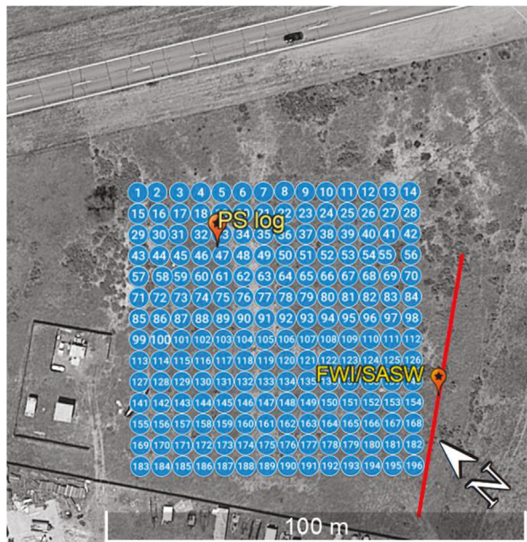
Figure 10. Plan view of the GVDA test site with the locations of several seismic testing (ANT, active-source FWI, and SASW) and PS log borehole. The blue circles represent the 196 3C 5 Hz nodal stations (this 3D ANT study), which were deployed in a 14 \times 14 grid at a uniform spacing of 5 m.
