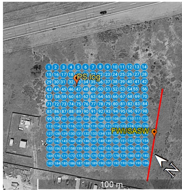
Figure 1. Plan view of the GVDA test site with the locations of several seismic testing boreholes and sensor arrays indicated. The blue circles represent the 196, 3-component, 5-Hz nodal stations used for 3D ANT in the present study, which were deployed in a 14 x 14 grid at a uniform spacing of 5 m.
