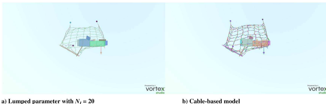
Fig. 18 Visual confirmation taken at t = 1.50 s of collision detection between net threads and smallest target geometry in simulation with a) N_I = 20 and b) cable-based model.
