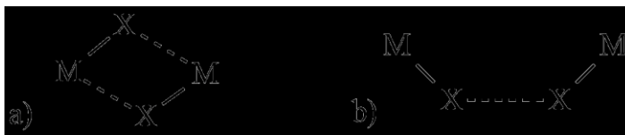
Scheme 1. a) The bihalide magnetic exchange pathway. b) The two-halide magnetic exchange pathway
