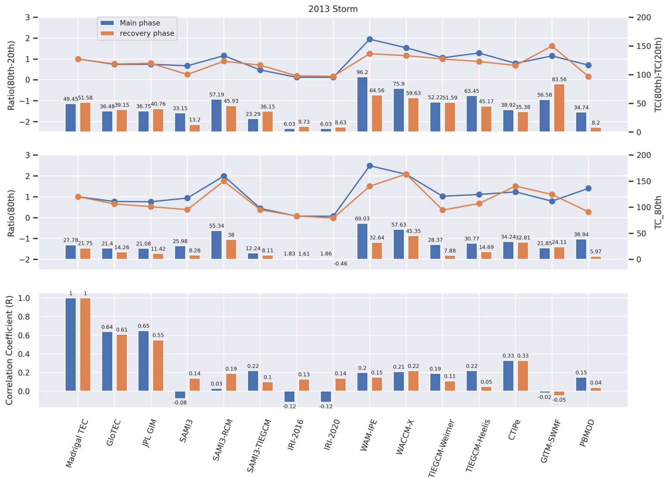
Figure 6. The ratios and correlation coefficient of total electron content change (TC). (top) The line plot and histogram denote the ratio of the TC difference from the 80th to 20th percentiles between models and observation ( \text{ratio}(80\text{th} - 20\text{th}) = \frac{(TC_M)_{80\text{th}} - (TC_M)_{20\text{th}}}{(TC_O)_{80\text{th}} - (TC_O)_{20\text{th}}} ) and the TC difference from the 80th to 20th percentiles ( ((TC)_{80\text{th}} - (TC)_{20\text{th}}) ). (middle) The ratios of TC at the 80th percentile and TC at the 20th percentile for each model. (bottom) Correlation coefficients of TC.
