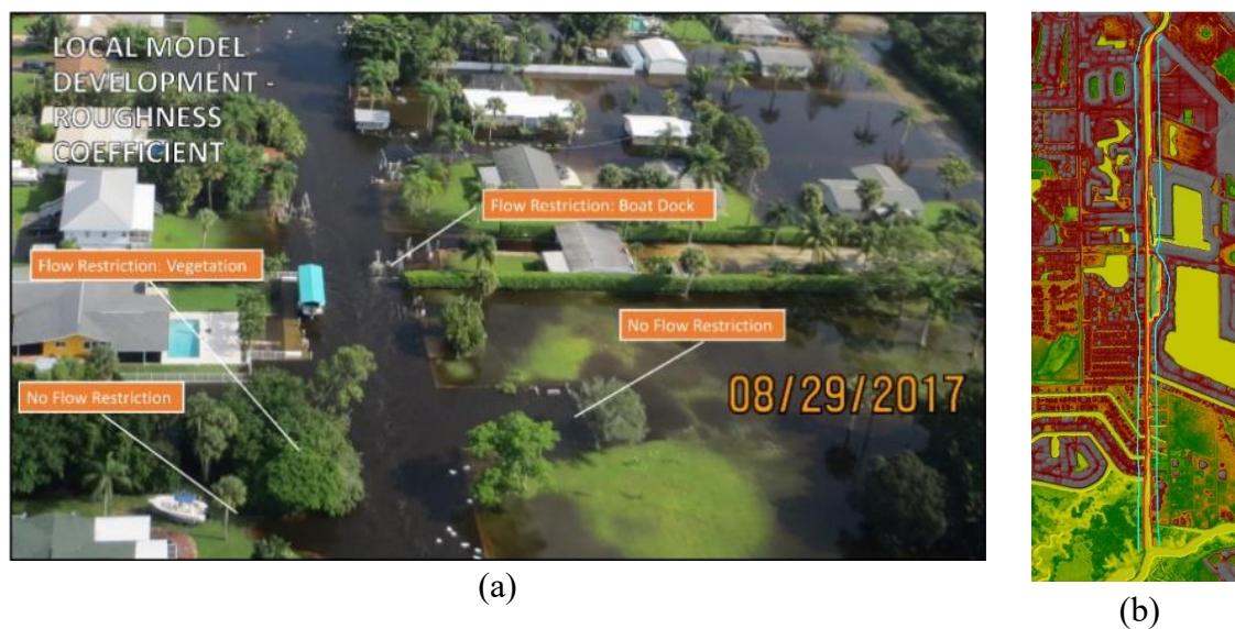
Figure 1. (a) Photograph of flooding situation during the stormwater event on 08/29/2017; (b) elevation map of the study area: Tenmile canal, FL
