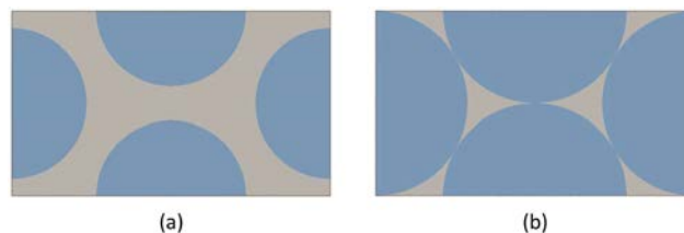
Fig. 6 Unit cells \mathcal{U} for hexagonal suspensions of monodisperse liquid 2-spherical inclusions of radius A at volume fractions (a) c = 0.6 and (b) c = 0.905 .
