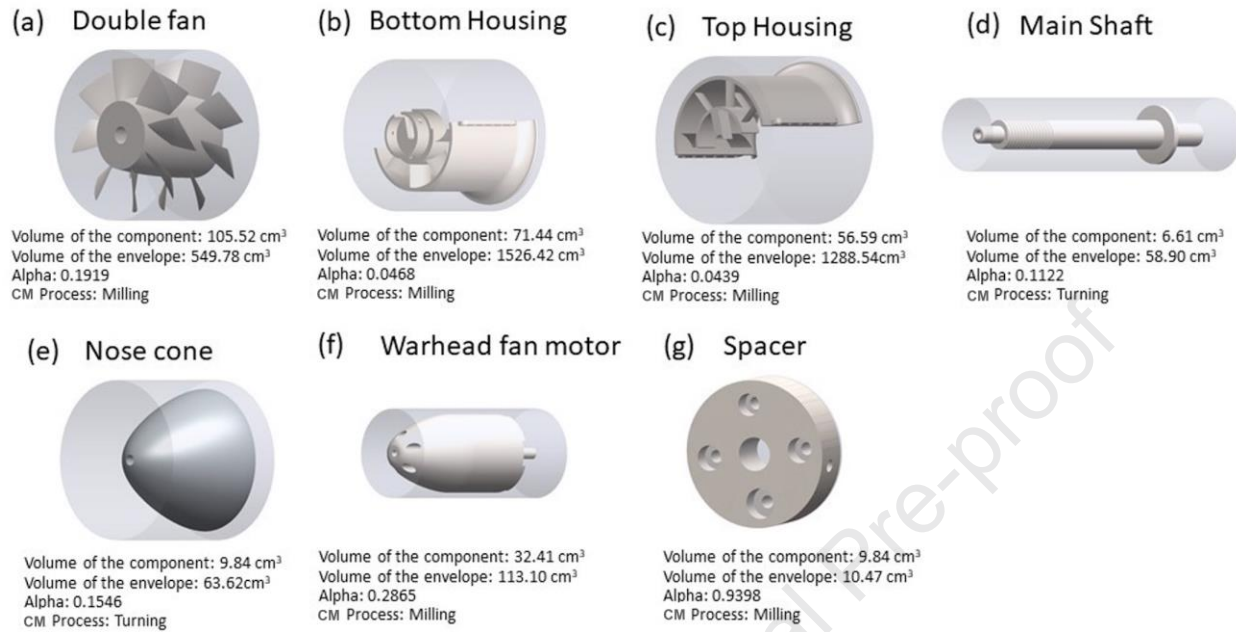
Figure 1. Details of each component's solid-to-envelope ratio (indicated by the value of Alpha) and manufacturing method. In order to produce the overall part, each component must be manufactured according to specialized CM methods, compared to a single additive method in the PBF process. Lower alpha values for larger components increases the likelihood for more energy efficient production in AM.
