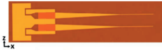
Fig. 23. Die microphotograph of the 180° waveguide bend structures without waveguide metallization for an equivalent waveguide outer bend radius of 100 \mu\text{m} .
