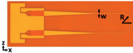
Fig. 20. Die microphotograph of the U-bend structures for the outer bend radius of 200\ \mu\text{m} and the waveguide width of 6\ \mu\text{m} .
