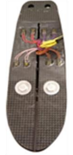
Fig. 4 Strain gauge assembly on prosthesis carbon foot.
