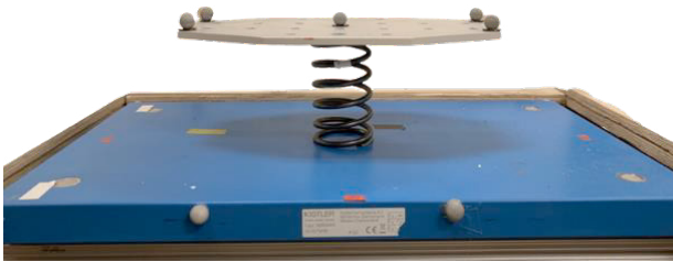
Figure 6. Validation test set up. Linear test spring has aluminum plate on top with markers. Blue force plate measures force reactions.
