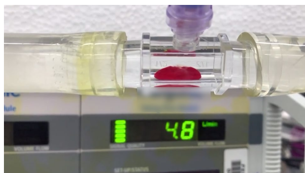
Figure 1. Blood clot formed in polycarbonate tube with flow probe screen in the background.
