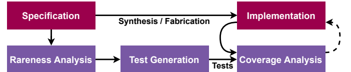
Fig. 2: Overview of test generation based Trojan detection
