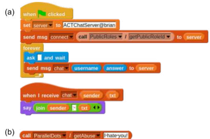
Figure 1: a) Completed client code for a chat app; b) An example RPC used to check if text is abusive.
