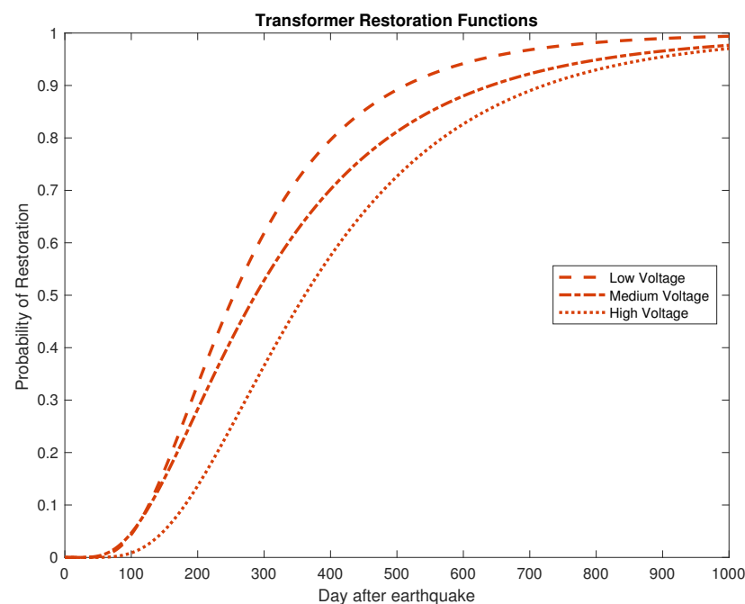
Figure 5. Transformer restoration functions, created with log-normal fit of survey data.
