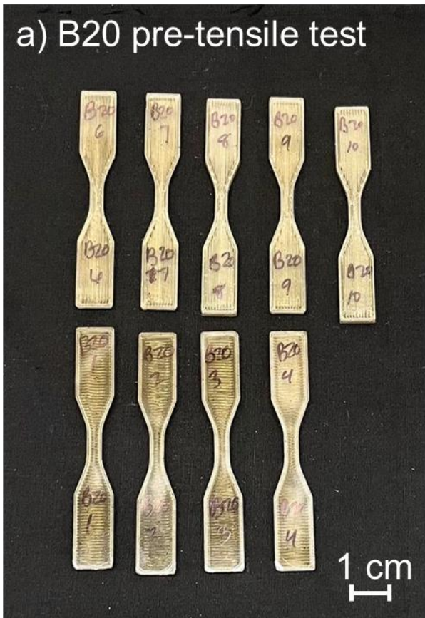
Figure S18. B20 samples 3D printed Type V tensile bars a) pre- and b) post-tensile test, bottom tests are 90° raster angle, top tests are 0° raster angle.
