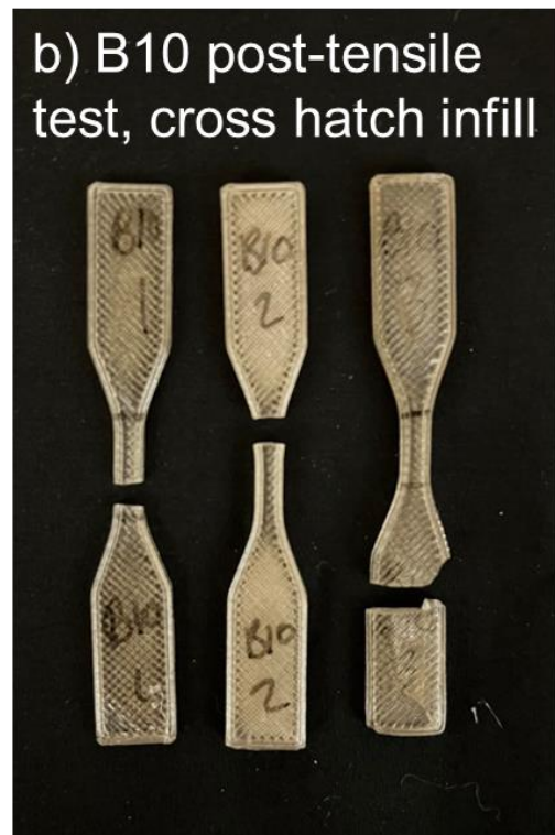
Figure S19. B10 samples 3D printed Type V tensile bars with a 45°/-45° crosshatching pattern a) pre- and b) post-tensile test.
