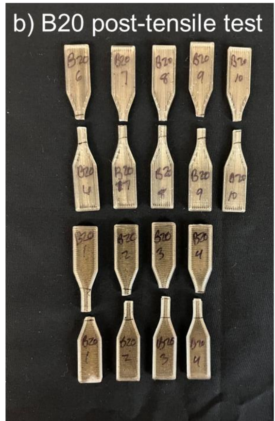
Figure S18. B20 samples 3D printed Type V tensile bars a) pre- and b) post-tensile test, bottom tests are 90° raster angle, top tests are 0° raster angle.
