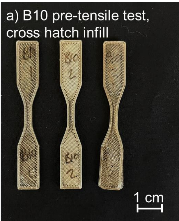
Figure S19. B10 samples 3D printed Type V tensile bars with a 45°/-45° crosshatching pattern a) pre- and b) post-tensile test.
