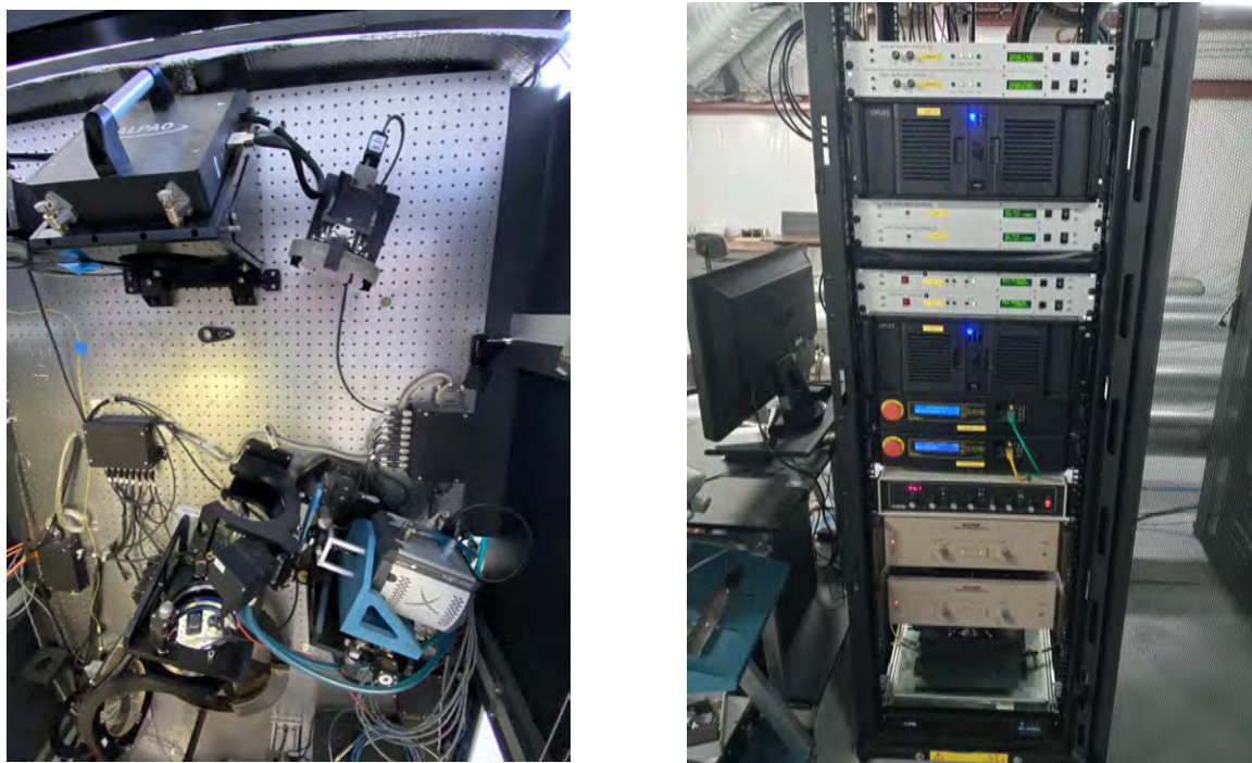
Figure 8: Left: The upper part of one of the AO benches with the DM at top and WFS at lower right. Right: The computer rack that controls two of the delay lines. At the very top are the 1U embedded system components which deal with the metrology signals. The black 4U components are the Linux computers which link the delay line control hardware with the rest of the CHARA Array control system. The two sets of two 1U embedded system components between the two computers are the voice coil interface (the upper set), and the stepper motor supervisor and limit switch interface (the lower set). Below the two components with the large red buttons are the reused components described in the text.
