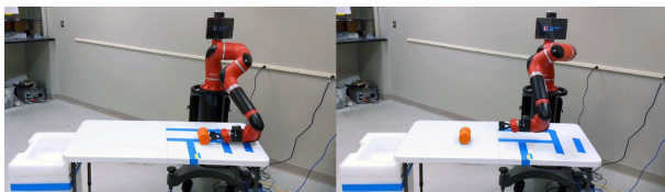
Fig. 9: Experimental setup for the cylinder rolling task. The cylinder is place at a designated starting point and the robot attempts to roll the cylinder into the basket at the end of the table.
