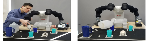
(a) Kinesthetic teaching of the (b) Yumi robot performing tea-making task to a Yumi robot. Adding Milk action.
