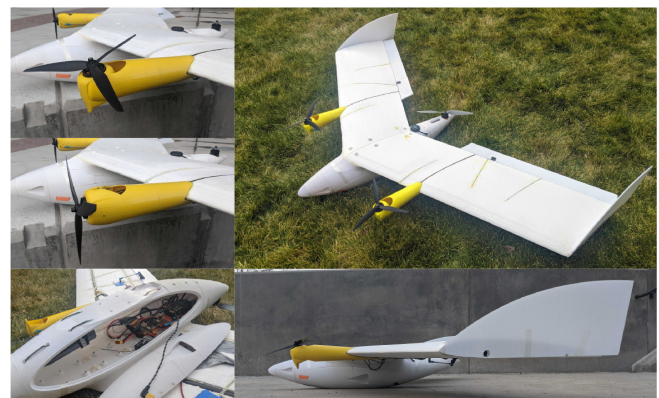
Fig. 8. Gannet assembled experimental prototype: Current iteration is mechatronically complete and flight-proven.
