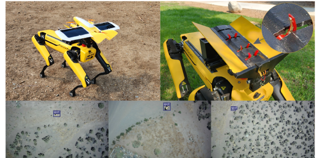
Fig. 7: Multi-day solar-powered recharging sequence with overnight hibernation.
