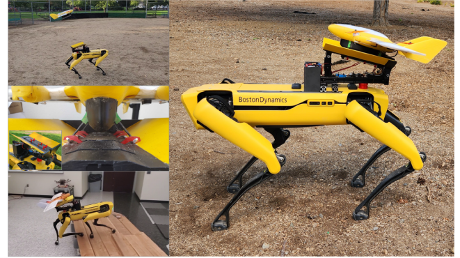
Figure 1: The Flexible Aerial / Legged Marsupial Autonomous (FALMA) system. Detail: The Docking & Recharging Backpack (DRB) design facilitating repeated deployment cycles, in situ fast-recharging on the go, and stable marsupial docking during aggressive legged locomotion.
