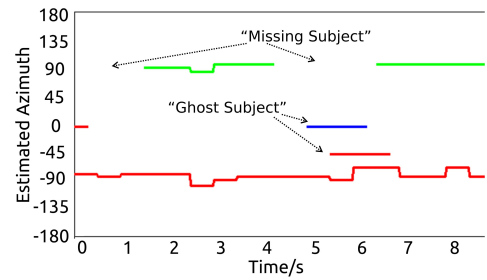
Figure 9: An example where SSL failed to reliably locate sound sources.
