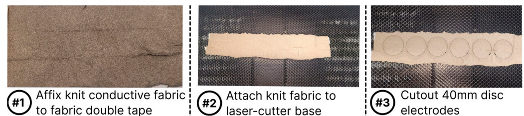
Figure 4. Laser cutting process used to create circular knit electrodes (E7).
