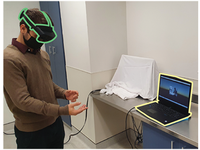
Figure 2: MR system overview for CVC placement. The local operator (left image) places a CVC while being assisted from a remote expert (right image) using the real-time mixed-reality communication system. We highlight the hardware components of the system.
