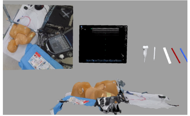
Figure 4: Remote view. The remote virtual workspace consists of the volumetric view (bottom center), the video feed (left), the ultrasound feed (top center), and the virtual objects (right). The virtual workspace can be placed in any room.
