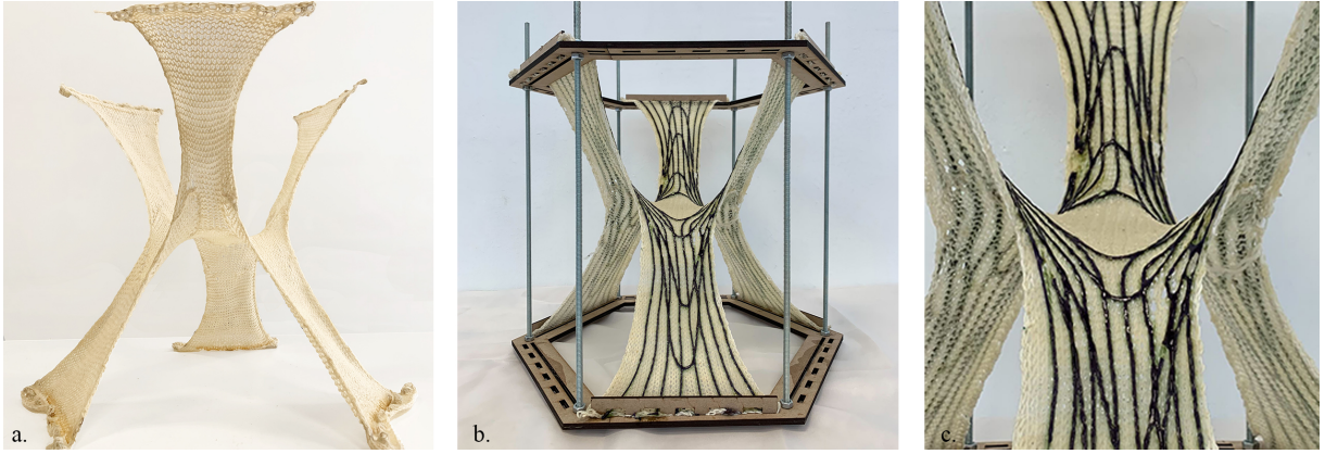
Figure 1: Biomaterial-based Stiffening of the knitting samples,
