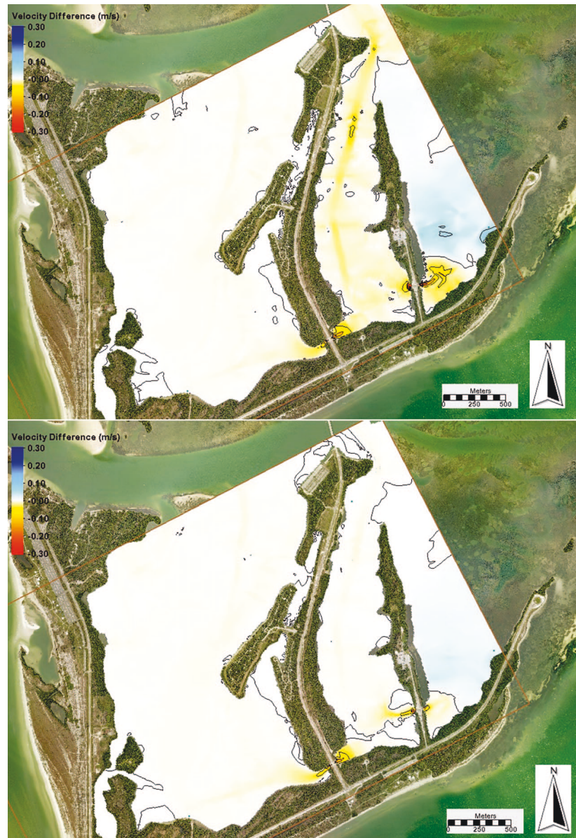
Figure 6. Flow difference map: both bridges closed minus existing conditions (A1–A2), positive value indicates stronger flow under the A1 condition, negative indicates weaker flow. Upper panel: under a peak ebb flow condition; lower panel: under a peak flood flow condition.
