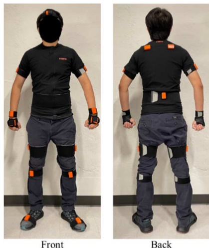
Fig. 1. Pictures showing the motion capture sensors setup.
