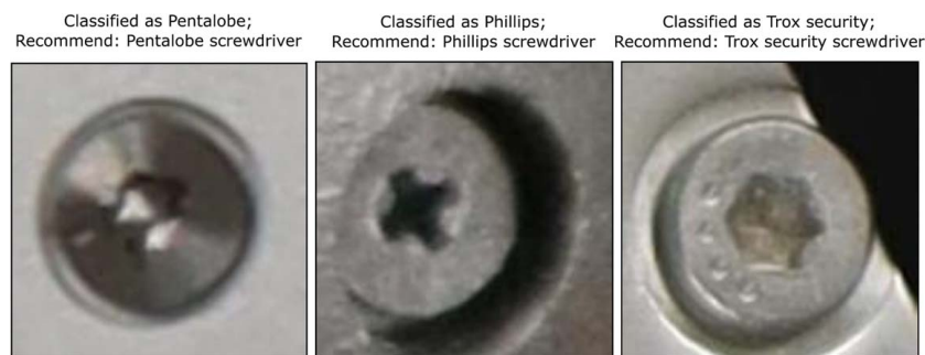
Fig. 8 Screw-type identification and tool recommendation results
