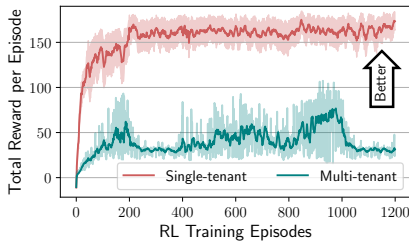
Figure 4: Training curves of the single-agent RL (for function Primes) in single- and multi-tenant environments.
