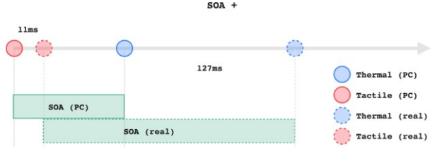
Fig. 2. Schematic illustration of the relationship between the SOA specified in the PC program and the SOA on the skin when a positive value is assigned to the SOA, accounting for computer response and delays.
