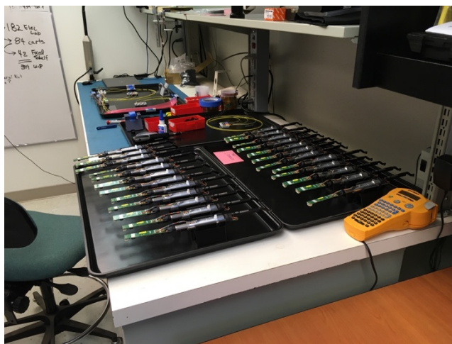
Figure 5: Production fiber positioner robots being prepared for optical fiber assembly integration at OSU.
