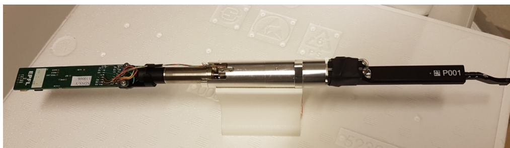
Figure 4: First-article fiber positioner robot fabricated by MPS Faulhaber in the AstroRobotics lab at EPFL.
