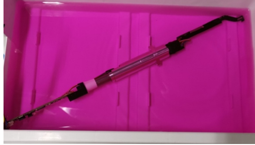
Figure 11. Fully powered-on robotic fiber positioner drowning in water/glycol coolant.
