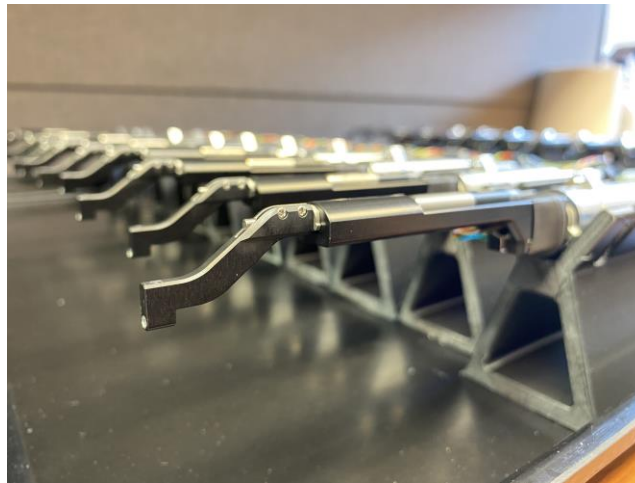
Figure 1. Fiber positioner robots with beta arm shown at the furthest extent and alpha arm extending just below two screws fixing the beta arm to alpha arm.
