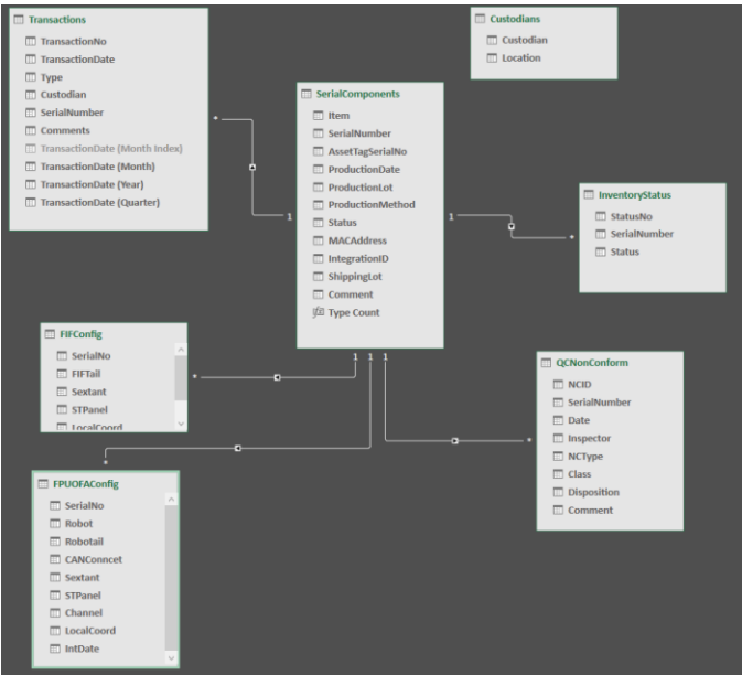
Figure 9. Simplified MRP data model using MS Excel data modeling tools. Tables and relationships are created to manage inventory, configuration, and quality data items and provide traceability for serialized components.
