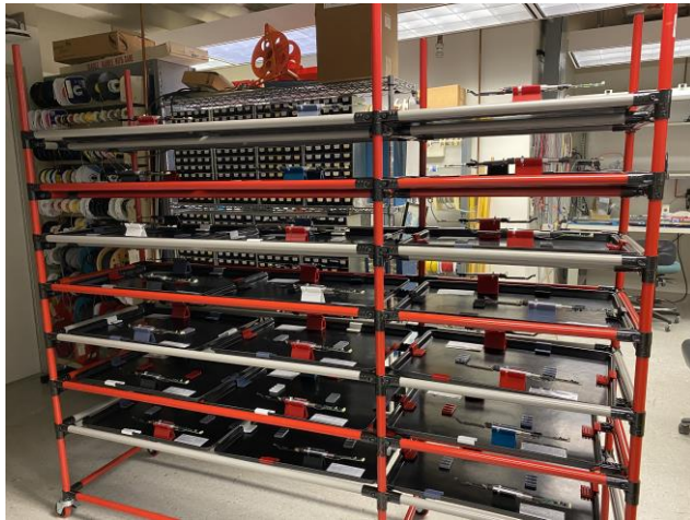
Figure 4. Specialized handling carts and fixtures. Left: FPR-OFA assembly WIP inventory cart used to move completed assemblies between work cells. Right: FPR fixture with base and clip used during FPR-OFA assembly and fixation.
