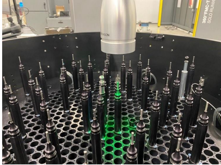
Figure 10. Optical probe on Hexagon CMM measuring a fiducial fiber core
