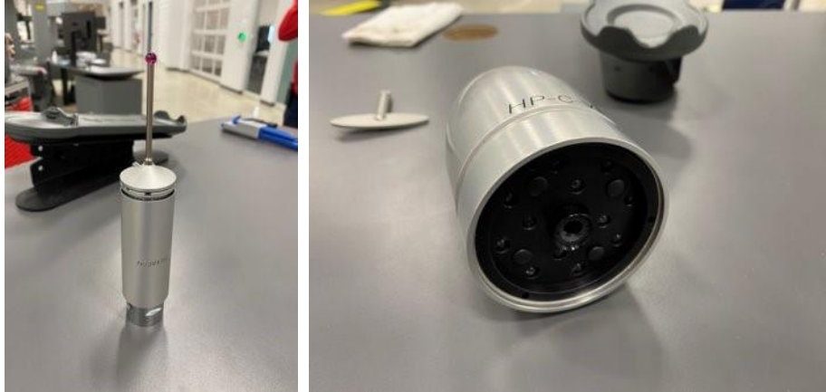
Figure 6. CMM Probes used for wok-mounted FIF metrology. Left: touch probe. Right: optical probe
