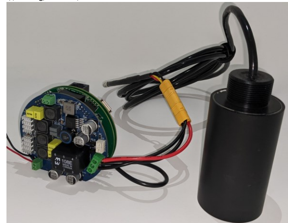
Figure 1: Photo of BlueBuzz with paired transducer. View is of computer board. The analog board and amplifier board are stacked behind.
