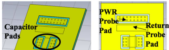
Fig. 3. Test fixture for a 3-terminal capacitor (left), and de-embedding fixture (right).
