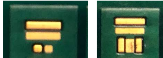
Fig. 4. Manufactured 2-terminal (left) and 3-terminal (right) test fixtures.
