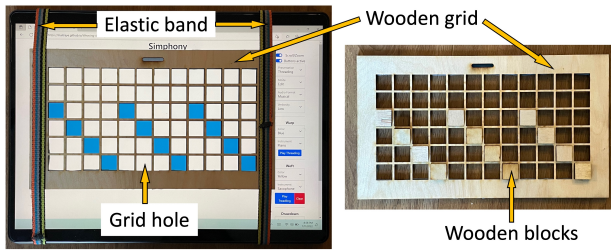
Figure 6: Left: A wooden grid is secured on top of the tablet showing the enlarged threading sequence of a twill pattern on Simphony. Right: The same threading sequence is created with wooden blocks on a standalone grid.
